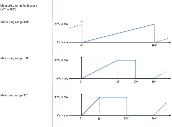
Default Setting: Output signal rotation cw (clockwise) with a view to the shaft.
